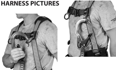
**Web Keepers:** DeWALT harnesses are provided with web keepers that serve to control the loose ends of the straps. These loose ends of straps, if left uncontrolled, can get caught in machinery or cause accidental disengagement of an adjuster. Hence, the user must ensure that there are no loose ends of the straps, and that these are kept in place by the web keepers.
