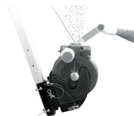
Potential water intrusion through cable opening of block casing.
