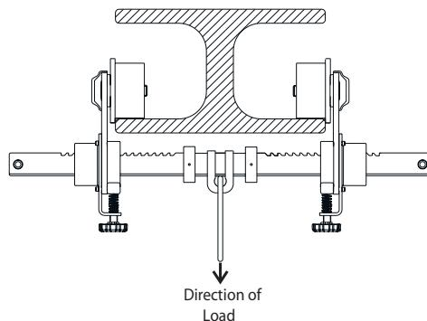
**Beam Anchor Trolley** is intended to be installed on flanges of beam from 9.84" - 3.14" (250mm-80mm) width.
