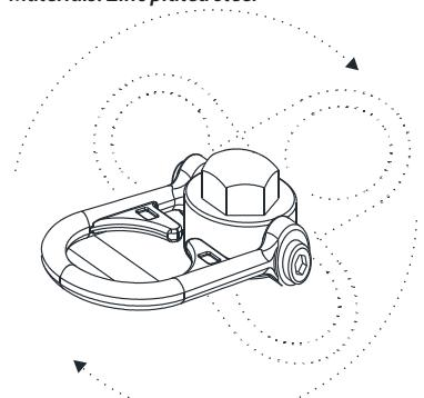
Single Point Swivel Anchor for Concrete Structure
