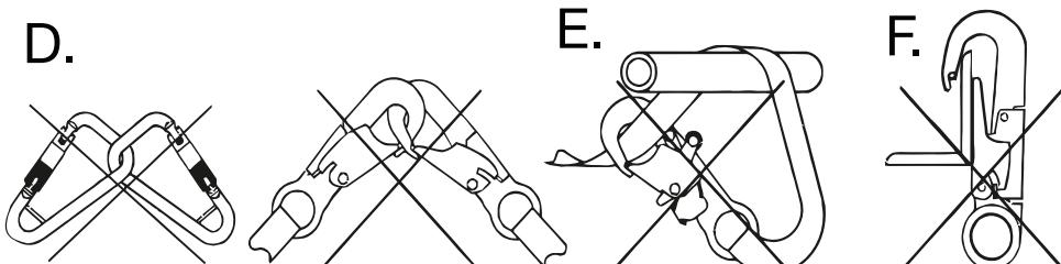
**⚠ WARNING:** If the connecting element to which a snap hook (shown) or carabiner attaches is undersized or irregular in shape, a situation could occur where the connecting element applies a force to the gate of the snap hook or carabiner. This force may cause the gate (of either a self-locking or a non-locking snap hook) to open, allowing the snap hook or carabiner to disengage from the connecting point.
