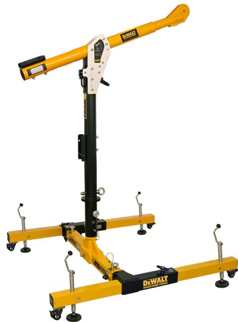
**ADJUSTABILITY:** Davit System Boom comes with 3 adjustment positions for the user to adjust the height to meet various situations: Min. Height: 65 in. (1.58 m) with 36 in. (0.91 m) offset. Middle Height: 79 in. (2.0 m) with 33 in. (0.84 m) offset. Max. Height: 90 in. (2.3 m) with 26 in. (0.66 m) offset.
