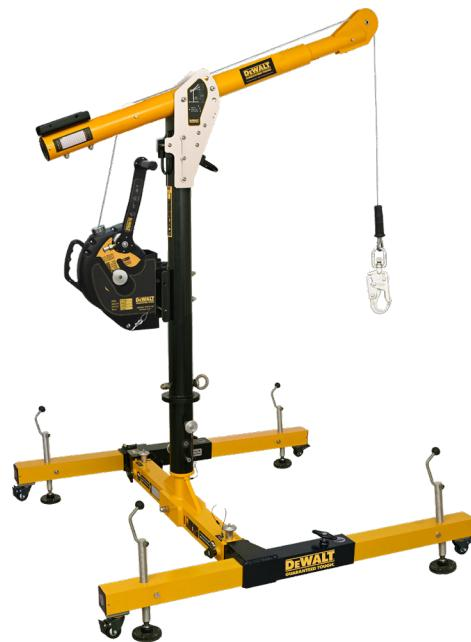
**ADJUSTABILITY:** Davit System Boom comes with 3 adjustment positions for the user to adjust the height to meet various situations: Min. Height: 47 in. (1.2 m) with 36 in. (0.91 m) offset. Middle Height: 61 in. (1.5 m) with 33 in. (0.84 m) offset. Max. Height: 72 in. (1.8 m) with 26 in. (0.66 m) offset.
