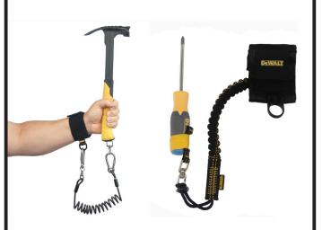
Anchorages - The final component of the system is anchorages and holders. The key variable in selecting the appropriate anchorage is the weight. Tools weighing 5 lbs. (2.3 kg) or less may be attached to the body. This can be done by securing the connector end to anchors like a tool holder, wristband or a secure point on the user's tool belt or harness. For all tools greater than 5 lbs. (2.3kg) the user must secure the connector end to a anchorage point rated for at least the weight of the tool.
