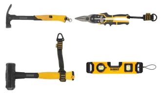
**Drop Prevention System** - In order to protect workers from injury and equipment from damage it is essential to select all components of a drop prevention system to securely attach tools and prevent accidental drops. The three main components of a system are attachment points, connectors such as tool lanyards, and anchorage points.
