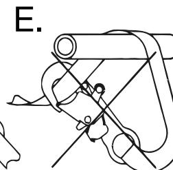
**⚠ WARNING:** If the connecting element to which a snap hook (shown) or carabiner attaches is undersized or irregular in shape, a situation could occur where the connecting element applies a force to the gate of the snap hook or carabiner. This force may cause the gate (of either a self-locking or a non-locking snap hook) to open, allowing the snap hook or carabiner to disengage from the connecting point.
