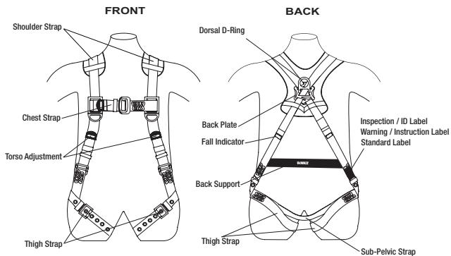
DeWALT full body harnesses are to be used as components in personal fall arrest, restraint, work positioning and rescue systems. The full body harnesses included in this manual conform to ANSI Z359.11-2021, and OSHA. Full body harnesses made of heat resistant webbing should be used when working with tools, material and environments of high temperature (e.g. foundries, welding, fire services, steel fabrication, oil industry, etc.).
