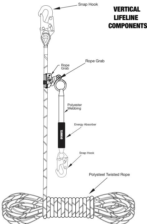
**⚠ WARNING:** Any equipment has been subjected to a fall should be removed from service.
