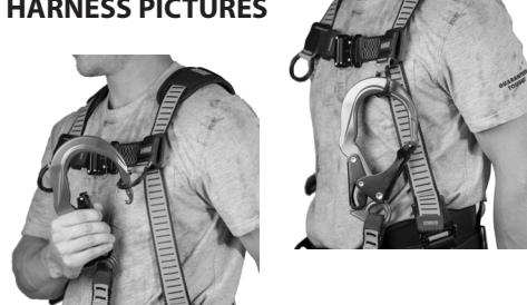
**Web Keepers:** DEWALT harnesses are provided with web keepers that serve to control the loose ends of the straps. These loose ends of straps, if left uncontrolled, can get caught in machinery or cause accidental disengagement of an adjuster. Hence, the user must ensure that there are no loose ends of the straps, and that these are kept in place by the web keepers.
