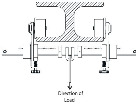
**Beam Anchor Trolley** is intended to be installed on flanges of beam from 9.84 in. - 3.14 in. (250 mm-80 mm) width.
