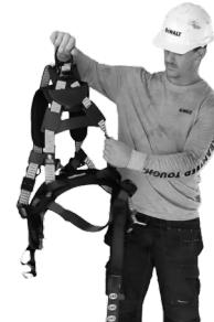
**STEP 1:** Lift up and hold the harness by the back D-Ring. Check to ensure that the straps are not twisted. (Fig. 1)
